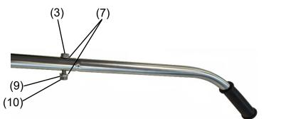
3) Insert the screws on the (4)tank holder Assembly and (5) carry assembly into the screw holes on (1) Pipe A, and fix them with the (7) plain washers, (9)spring washers and (10)nuts.
