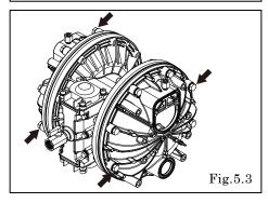
• Remove the 16 retainer bolts from the out chamber, and remove the out chamber. [Fig.5.3]
