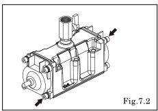
• Remove the 8 cap A and cap B retainer bolts, and remove cap A and cap B. [Fig.7.2]
