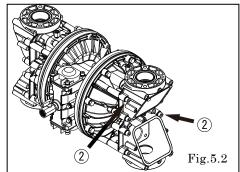
• Remove each 4 bolts ② from the valve case(in) and the valve case(out), and remove the valve case(in), the valve case(out), the O ring and the gasket. [Fig.5.2]
