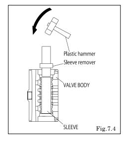
• Remove the sleeve using the sleeve remover (special tool: Part number 713180). [Fig.7.4]
