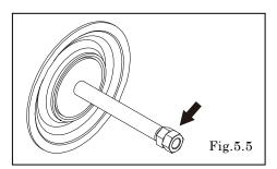
• Fix a double nut to one end of the center rod and take the diaphragm and center disk off the opposite end. [Fig.5.5]
