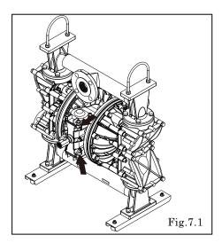
• Remove the 6 retainer bolts from the valve body, and remove the valve body. [Fig.7.1]
