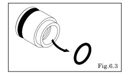
• Remove the packing from the throat bearing. [Fig.6.3]
