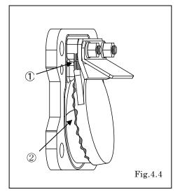
• If ① or ② are broken or cracked, replace it.
