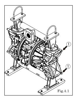
${\ }^{\bullet}$  Remove 4 bolts  ${\ }^{\textcircled{1}}$  from the cover, and remove the cover.  $[{\rm Fig.4.1}]$
