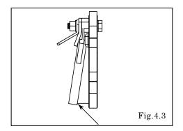
• If there is a gap between the flap valve and valve seat, replace it. [Fig.4.3]
