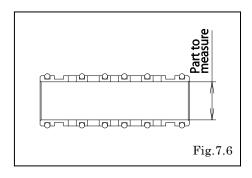
• Sleeve Assembly [Fig. 7.6] Measure the inside diameter, and if it is outside the usable range, replace the c spool valve assembly.
