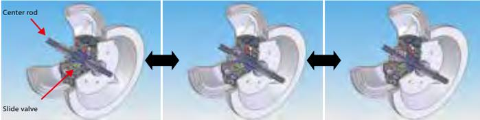
Mechanically-actuated air motor based on the diaphragm movement.
